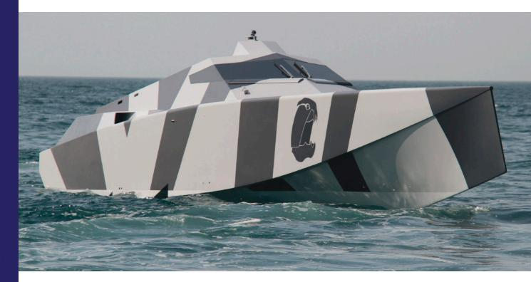
The WP18 Strike Craft is a sea proven Ultra High Speed Stealthy Assault and Special Operation Vessel. The WP18 stealthy design is characterized by a low visual profile, low radar cross section and low infrared signature.
