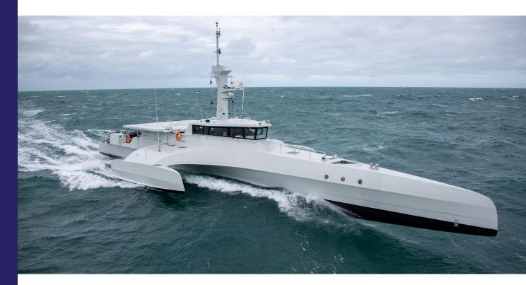
The sea proven OCEAN EAGLE 43 is an ocean patrol trimaran combining a very slender hull with two small floats designed to maintain the required stability.
