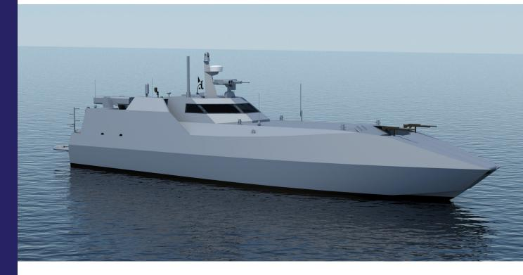
The HSAB 20 is part of the CMN's Sea Proven High Speed Interceptor Family. It is designed as a stealthly high-speed craft, able to perform the tasks required by a High Speed Assault Boat's mission profile.
