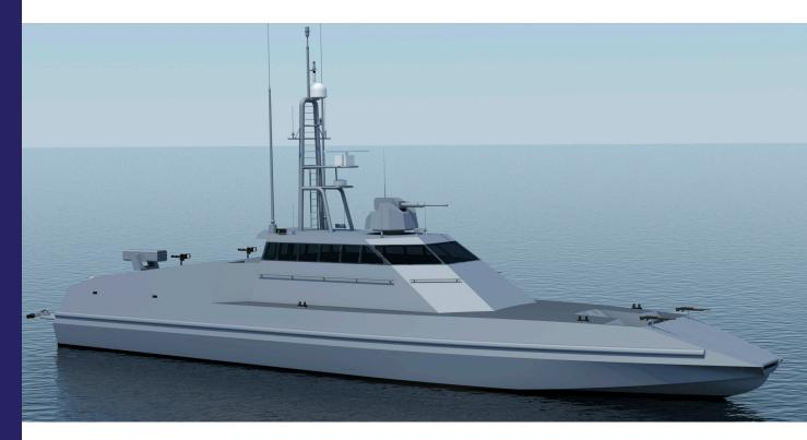
The HSAB 32 is part of the CMN's Sea Proven High Speed Interceptor Family. It is designed as a stealthly high-speed craft, able to perform the tasks required by a High Speed Assault Boat's mission profile.
